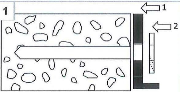
After preparing borehole (Annex B5, figure 1+2), position first fixture (1), then filling washer (2)
