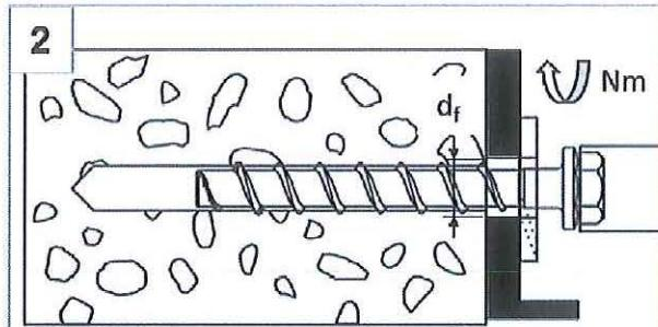
Install with torque impact screw driver
