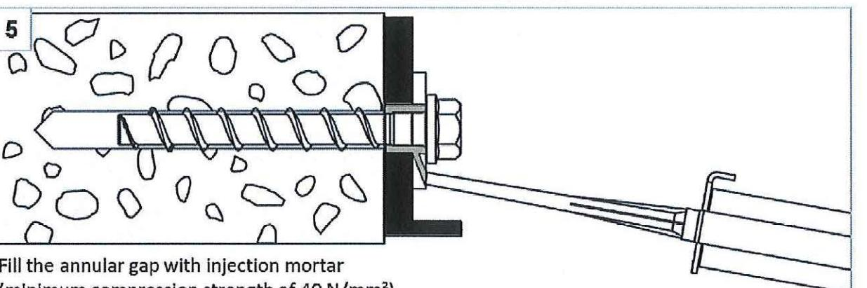
Fill the annular gap with injection mortar
